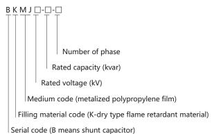
Note: The split phase compensation capacitor model is the product with suffix YN. For example, BKMJ 0.4-15-3YN means the line voltage is 400V, three-phase aggregate capacity is 15kvar, and the product inside is of star connection, zero conductor N is led out.
